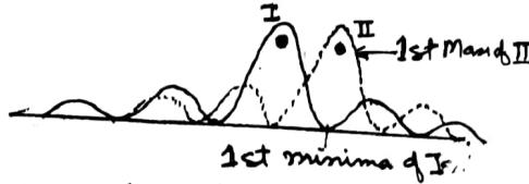
Two very close lying objects are said to be just resolved if the 1st Maxima of IInd object falls on the 1st Minima of 1st object or vice versa at the observers eye.
