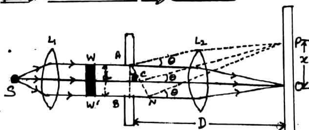
Consider a monochromatic light source S. Light from S is made parallel after refraction through lens L<sub>1</sub>, thereby forming a plane wavefront WW' which is incident on a slit AB of width 'd'. As per Huygens principle, each point of slit AB acts as a source of secondary disturbances/wavelets.
